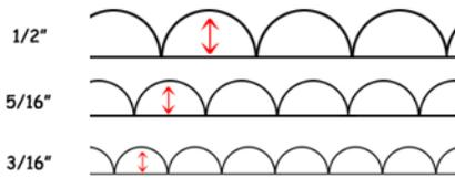
The length of each roll varies depending on which type of bubble. Small bubble has a length of 750 ft, medium bubble has a length of 375 ft and large bubble has a length of 250 ft.
